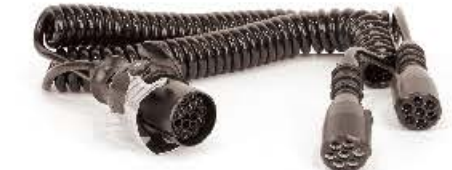
YW1130 Adaptor Double Spiral Coil With Molded Plug TPU Coil I.D. \phi 45mmx(6x0.75+1x1mm 2 ) Working Length:2x3M, Total Length:2x4M
